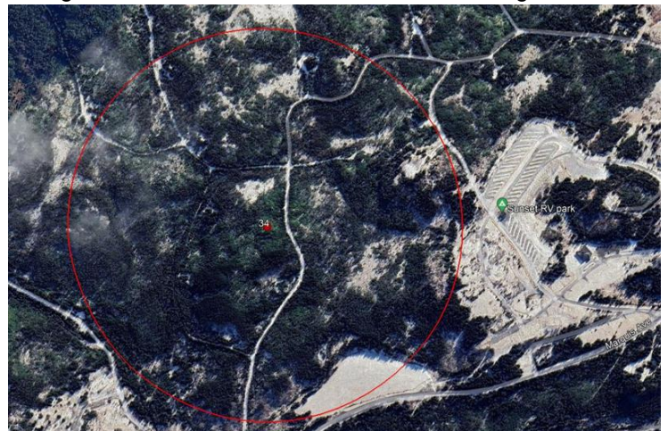
Figure 8 Wind Turbine #34 Maximum Ice Throw Distance if Hub Height and Rotor Diameter reduced to 105 m and 162 m, respectively
