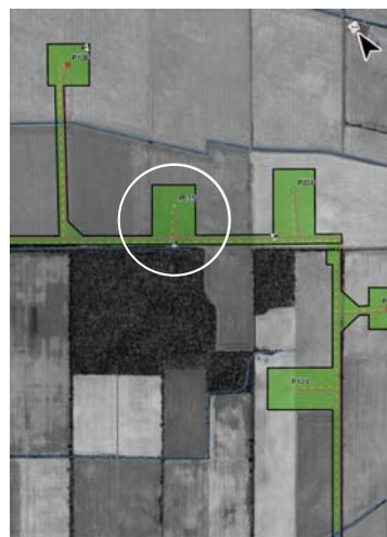
Planned temporary construction area showing turbine locations, access roads and collector lines
