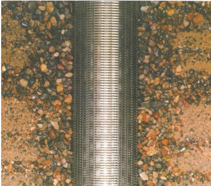
Figure 3: Illustration of natural filter formation around a well screen (from Driscoll, 1986, Figure 15.3)
