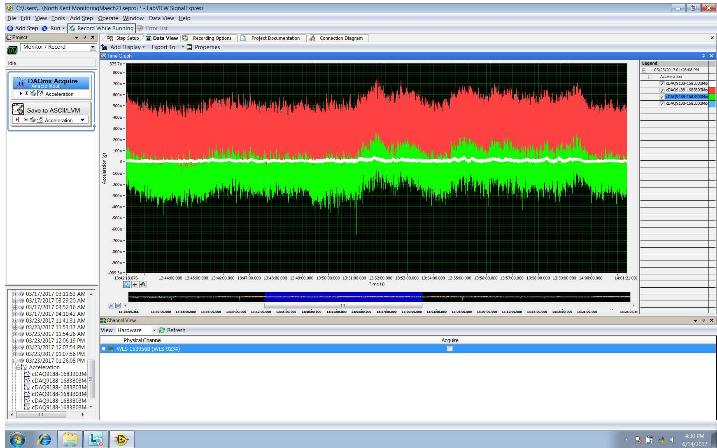
Figure I-15A: Acceleration Time History Detail, T42 Site, March 23, 2017 illustrating data from accelerometers installed within rock at borehole BH-103 during a quiet period in the absence of any site activities and in the absence of nearby traffic. Uniaxial accelerometer data shown in white, with triaxial accelerometer data shown in red (vertical), green (longitudinal) and blue (transverse) for the different orientations. Note that the different ranges of output are primarily related to the differing performance specifications of the two types of instruments. Accelerometer output, using the data logger used at this site, is shown in fractions of the gravitational acceleration constant g . The minimum and maximum values shown on the vertical axis are -989.3 \times 10^{-6} g and 875.7 \times 10^{-6} g ( micro-g as identified on graph axis with unit u ).
