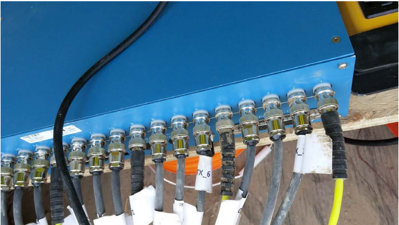
Photograph 11: Field connection of signal conditioner/power source.
