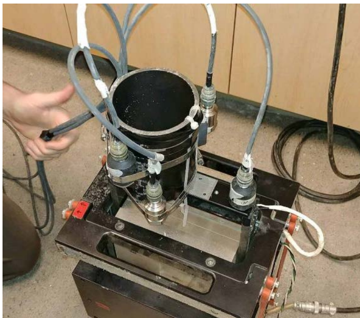
Figure G-1: Physical arrangement of shaker unit, pipe and four accelerometers prior to exposure to controlled vibrations.
