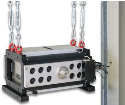
APS 420 with APS 8610 - Modal Stinger and APS 8612 - Steel Cable Kit prepared for Free Body Mode operation
