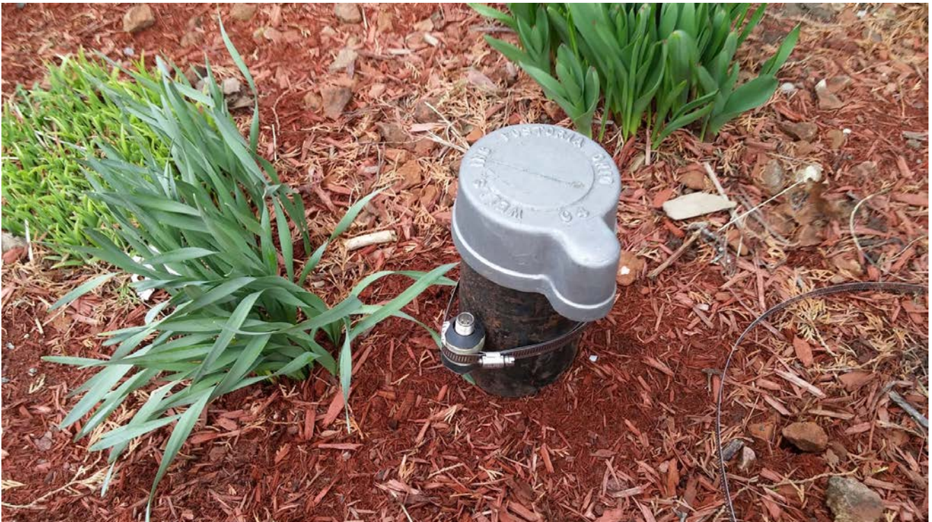
Photograph 30: Seismic accelerometer coupled to Well #1 casing.
