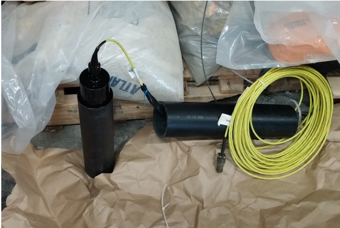
Photograph 7: Seismic accelerometer mounted on steel base of protective housing with connections coated with spray-plastic.
