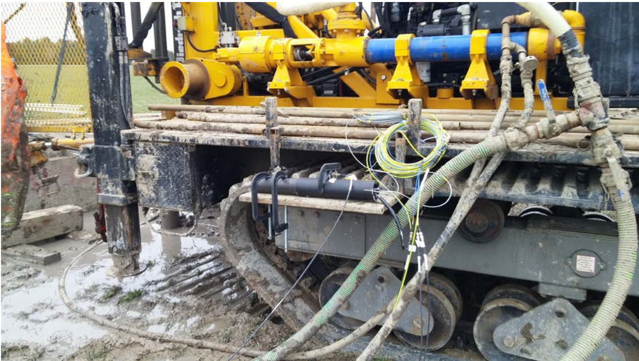
Photograph 15: Coupling of accelerometers in protective housing to drill rig, as vibration source, along with independent accelerometer field checked with controlled-source vibration measurement system (at T42 site).
