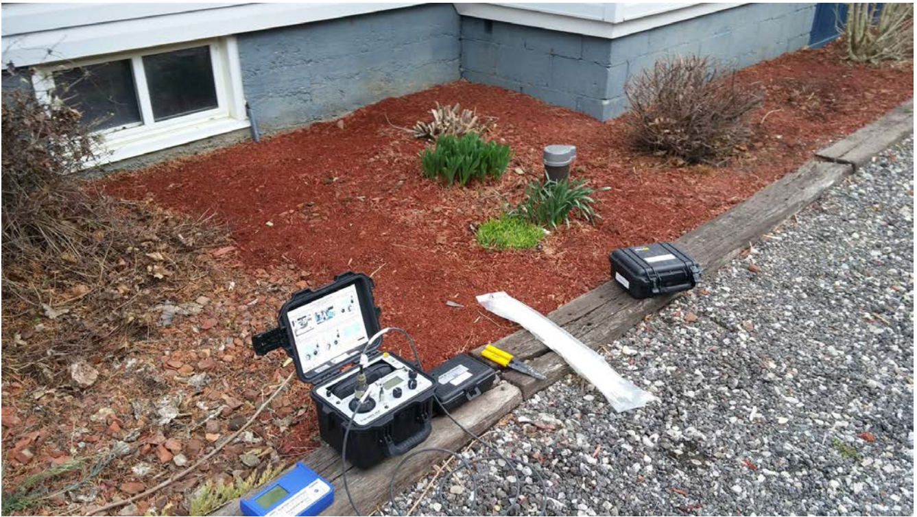
Photograph 29: Controlled-source vibration measurement system at Well #1 location.
