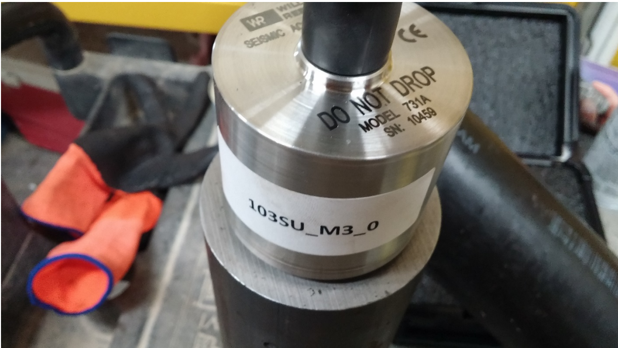
Photograph 6: Seismic accelerometer mounted on steel base of protective housing.
