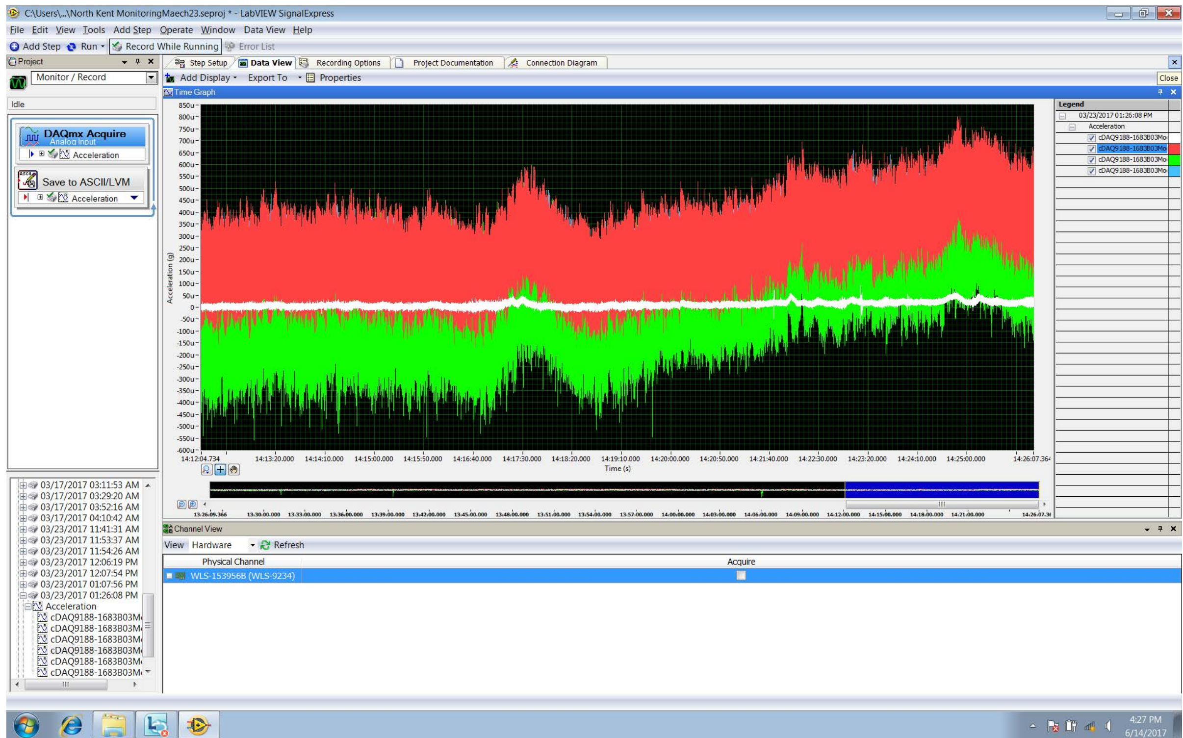
Figure I-15B: Acceleration Time History Detail, T42 Site, March 23, 2017 illustrating acceleration data obtained during a time period on the T42 test site on March 23, 2017 when the vacuum truck backed slowly along the wooden mats, passing borehole BH-103 at a distance of about 5 m, and started operating to remove soil cuttings and water from a bin located about 35 m from borehole BH-103. The minimum and maximum values shown on the vertical axis are -600 \times 10^{-6} g and 850 \times 10^{-6} g (micro-g as identified on graph axis with unit u).
