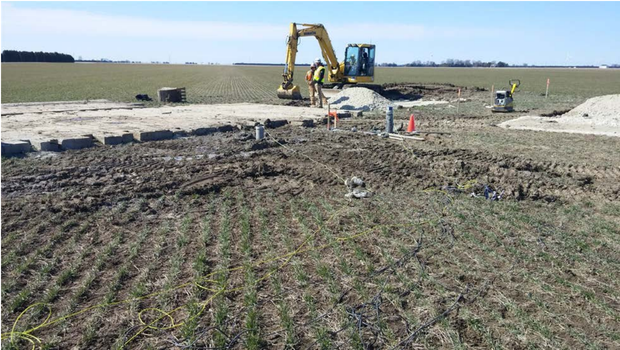
Photograph 21: Field set up of data loggers and signal conditioner systems at T42 site for testing of installed accelerometer systems with InstanTel Minimate data logger positioned temporarily on borehole casing and geophone placed nearby (looking toward test pile location).
