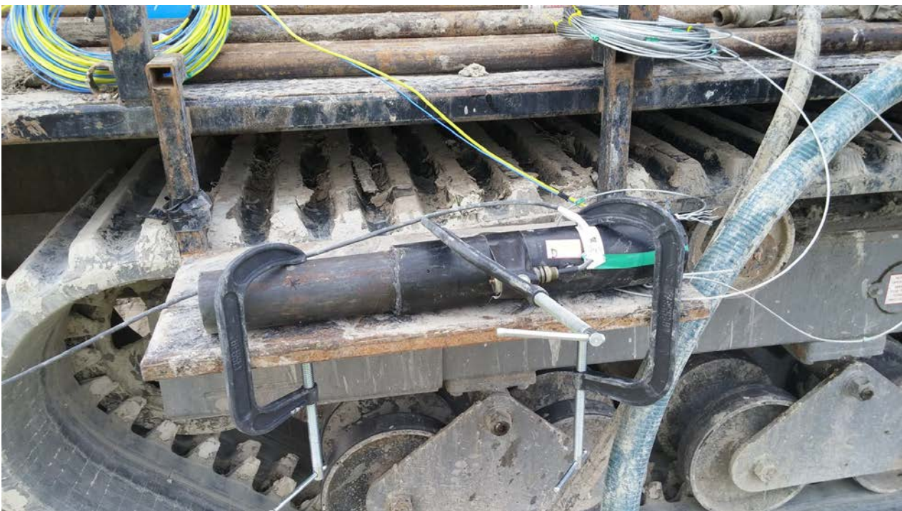
Photograph 16: Close-up view of coupled accelerometers in protective housing, drill rig and independent accelerometer (at T42 site).
