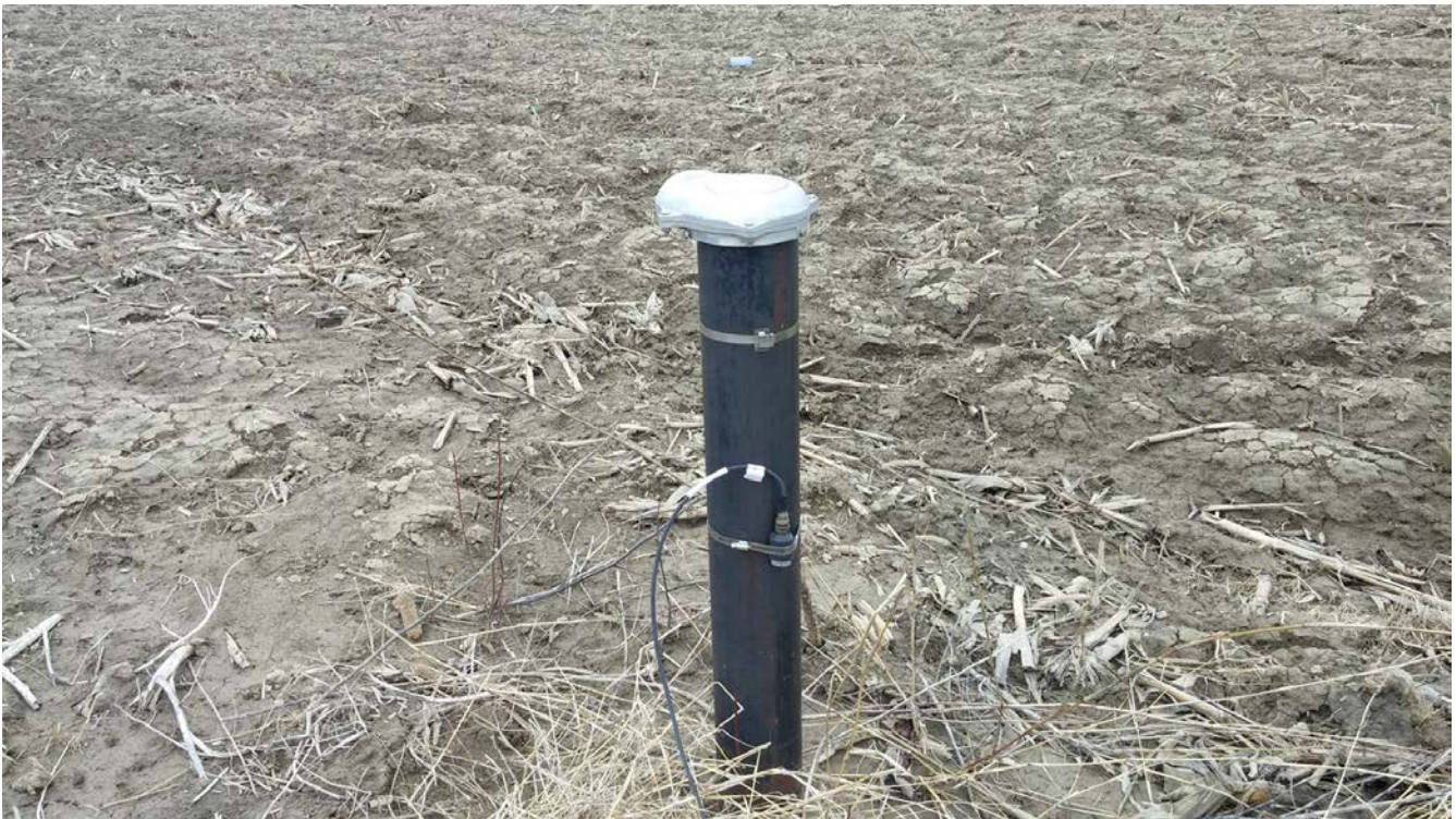
Photograph 32: Seismic accelerometer coupled to Well #2 casing.
