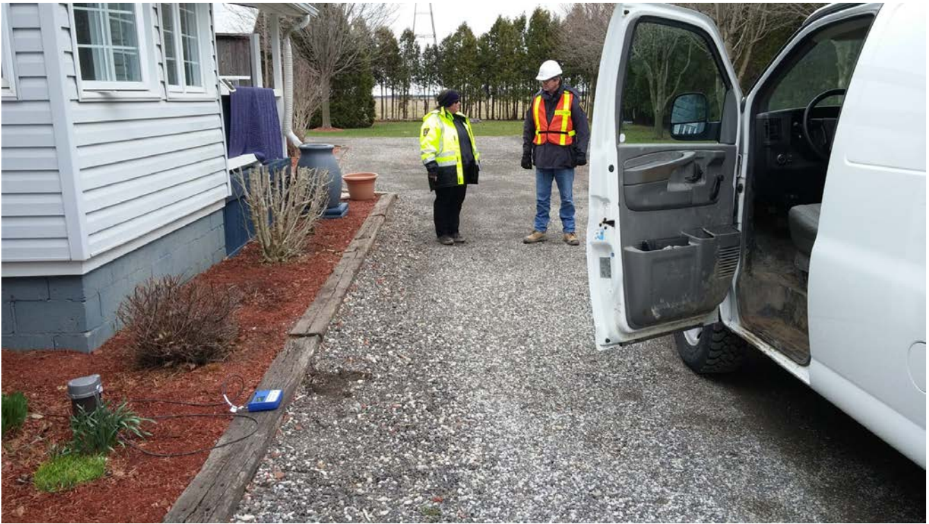
Photograph 31: Seismic accelerometer coupled to Well #1 casing showing data logger and Golder van.
