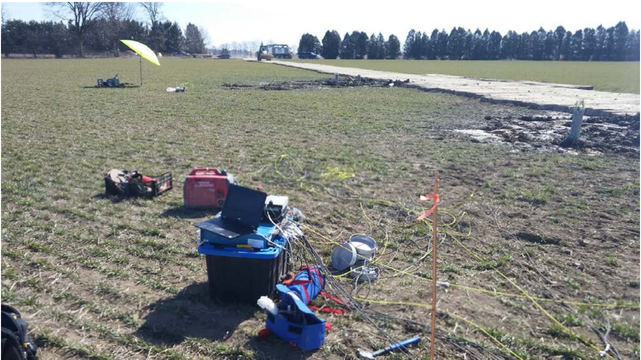
Photograph 20: Field set up of data loggers and signal conditioner systems for testing of installed accelerometer systems (looking toward Claymore Line) at T42 site.
