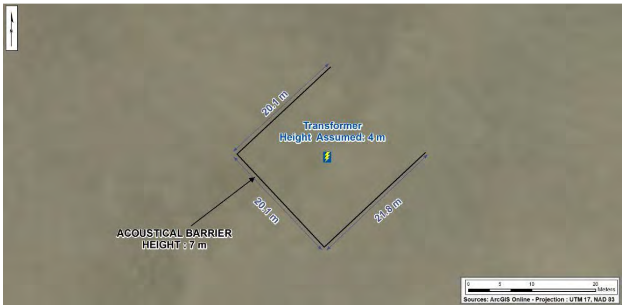
Figure 4-1 North Kent 1 Wind Project substation barrier
